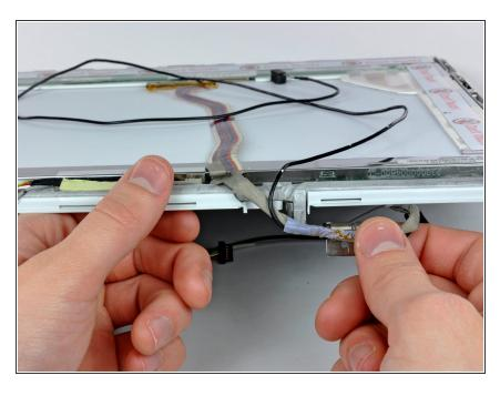
Remove the display data cable from the display.
