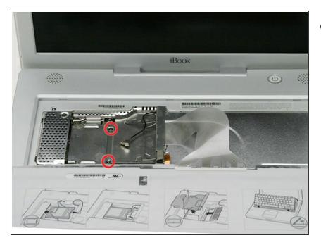
Remove the two Phillips screws that secure the RAM shield.
