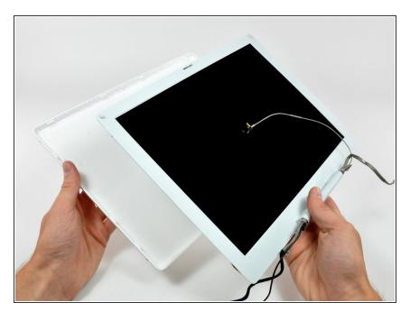
Lift the rear bezel off the display.
