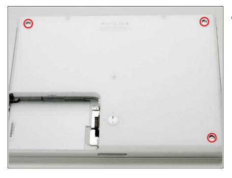
Remove the three newly-revealed Phillips screws.
