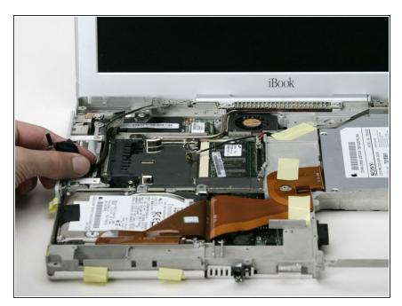
Deroute the display data and microphone cables, removing tape as necessary.
