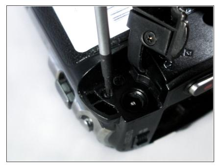
Pull out the charging port (DC input terminal) cover and remove the 4mm screw located next to the input terminal.
