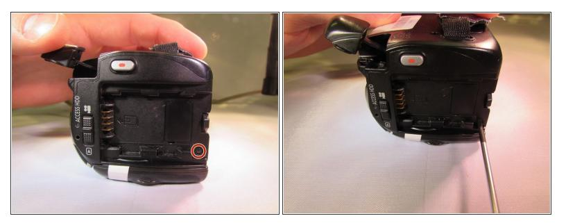
Remove the black 4 mm screw from the back of the camcorder underneath where the battery would have been.
