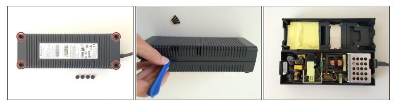
• After removing the 4 screws, pry along the edge to get the two halves separated
