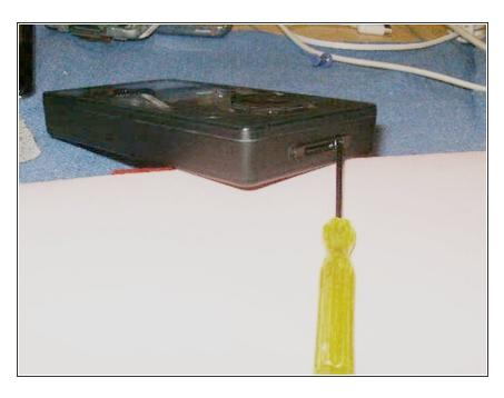
Start off by removing the spacer from the bottom dock port. It is just pushed in, so all you need is a small jeweler's screwdriver to pry it out. Use the smaller ends of the port as the pry point so you don't break the spacer.
