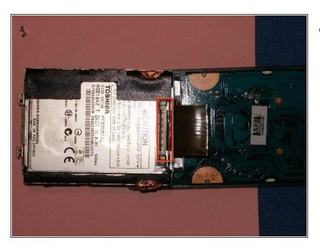
With the battery and the four screws for for the hard drive caddy removed, lift the caddy up and flip it toward the headphone end of the Zune. Remove the hard drive cable clip by opening the black clip on the connector. Use your fingernails or the iPod tool to move the clip carefully to the open position. Take off the sticky tape to reveal the hard drive bumpers. Remove them to free the hard drive. Now replace the hard drive and reassemble the Zune.
