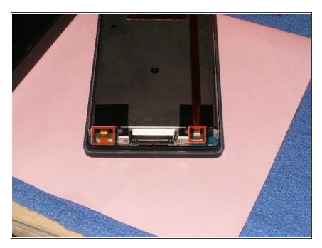
Disconnect the battery by lifting the brown slide gently up, freeing the cable. You can now safely remove the battery. Disconnect the clickwheel cable afterwards.
