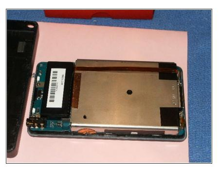
Now with the backing off we have free access to the battery and the hard drive caddy.
