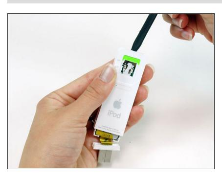
Continue to slide the iPod out of its casing by using a spudger to push on the logic board near the headphone jack.
