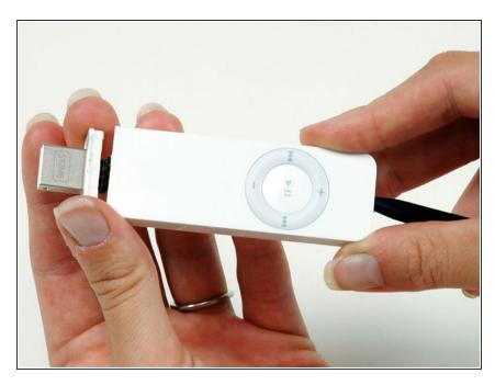
After the USB port comes free, carefully slide it out of its housing.
