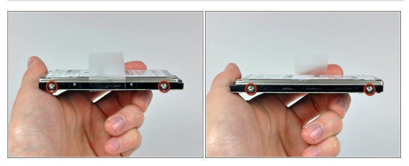
Remove the two T6 Torx screws from each side of the hard drive (four screws total).
