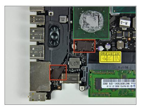
Peel off the tape covering the microphone cable connector and left speaker cable connector.
