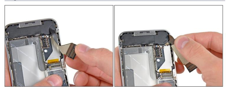
• Carefully peel the dock ribbon cable off the logic board and the lower speaker enclosure.
