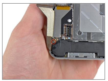
Remove the 1.9 mm Phillips screw securing the bottom of the logic board to the inner case.
