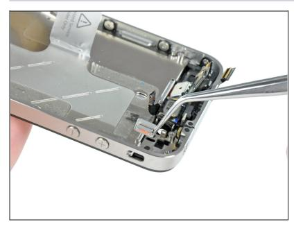
• Remove the vibrate/ring switch from the outer case.
