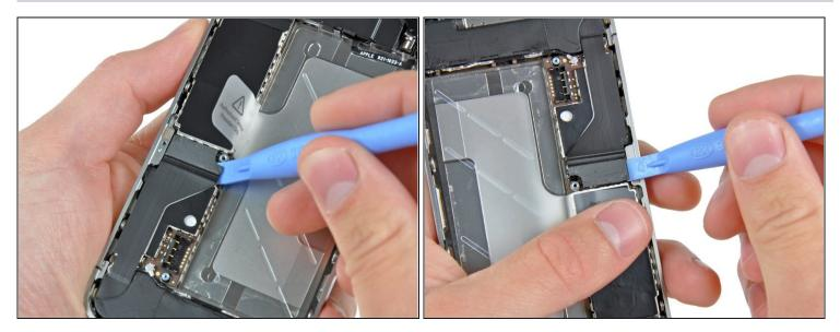
• Use an iPod opening tool to gently pry the dock cable connector up off the logic board from both short ends of the connector.
