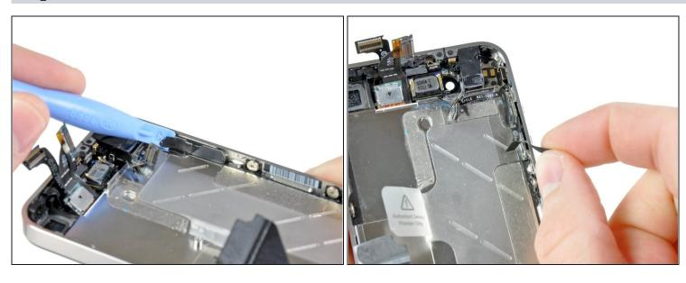
Use the edge of a plastic opening tool to peel the small strip of black tape off the back of the volume button bracket.
