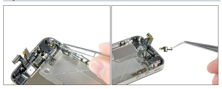
• Use a pair of <u>tweezers</u> to carefully pull the silent switch and its bracket from the side of the outer case.
