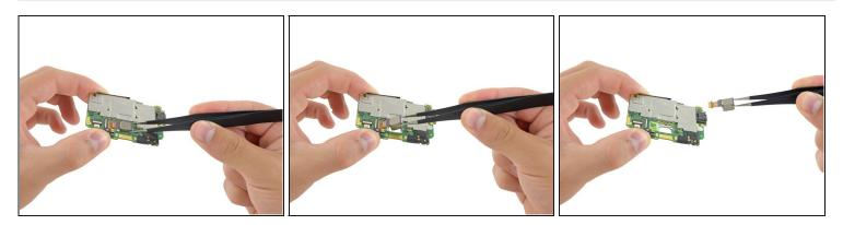
• Use tweezers to lift and remove the rear camera from the logic board.
