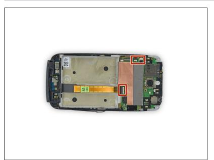
Repeat the procedure from steps 19 and 20 to remove the cables from the remaining ZIF connectors.
