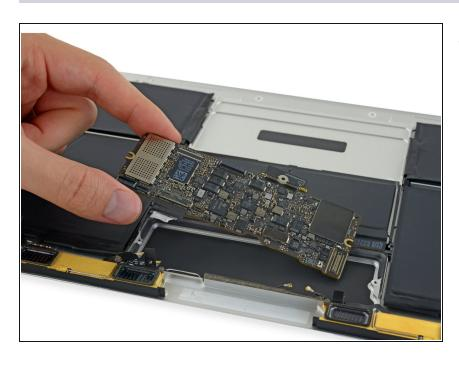
Remove the logic board.
