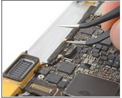
• Insert one arm of your angled tweezers under the metal neck of the first antenna connector and pry up to disconnect it.
