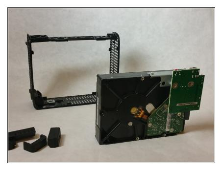
Remove all the rubber pieces from the four corners to unhinge the motherboard.
