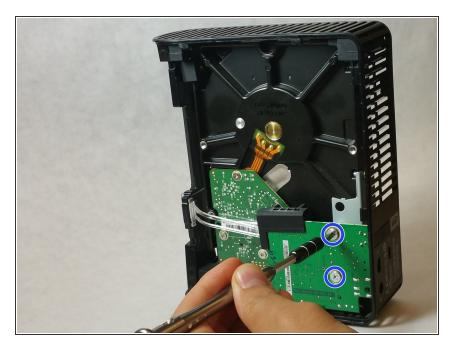
Unscrew the two screws from the motherboard.
