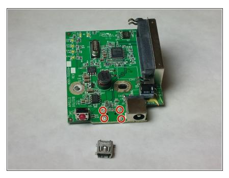
Grab the mini USB port and align it with the appropriate metal docks on the motherboard.
