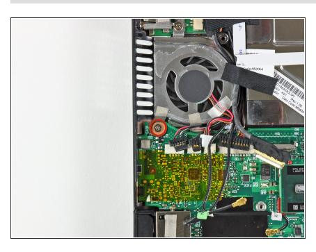
Remove the single 4.5 mm Phillips screw securing the motherboard to the lower case near the fan.
