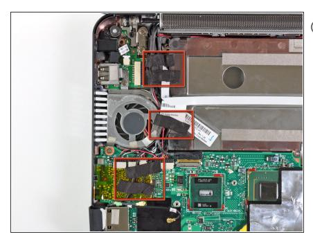
if present, remove the several pieces of black cloth tape securing the cables to the upper case near the fan.
