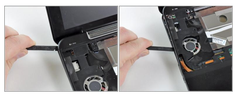
Repeat the same procedure as mentioned in the previous step to release the clips along the left side of the upper case.
