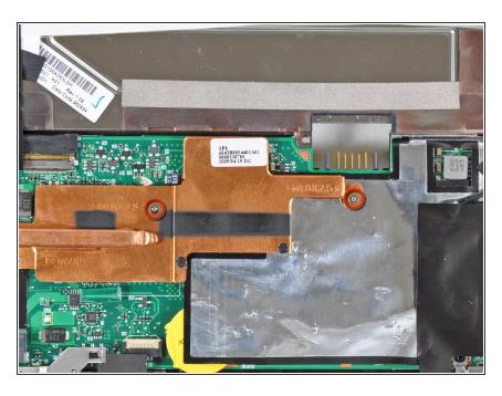
Remove the two 2.5 mm Phillips screws securing the heat sink to the motherboard.
