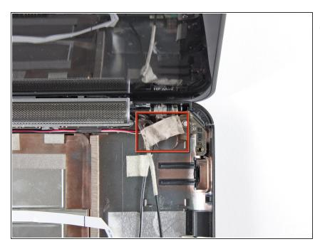
i If present, peel back the strip of white cloth tape highlighted in red to reveal a display screw.
