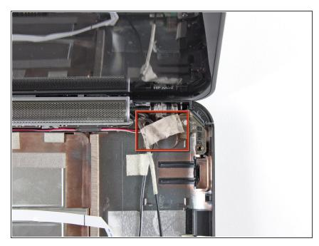
if present, peel back the strip of white cloth tape highlighted in red to reveal a display screw.
