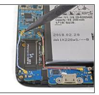
Use the pointed edge of a spudger to disconnect the Bluetooth and Wi-Fi antenna cable connectors from their sockets on the motherboard.
