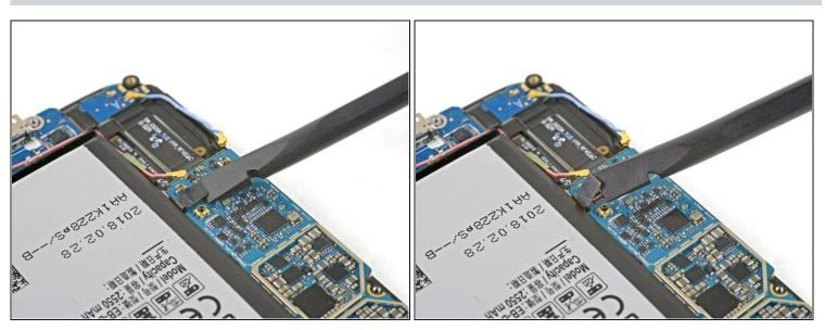
Use the flat end of the spudger to disconnect the home button connector.
