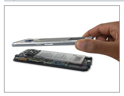
Lift the midframe assembly up to separate it from the rest of the phone.
