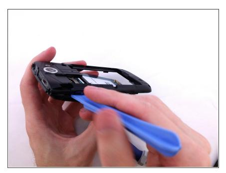
With plastic opening tool continue prying around the edge of the back assembly.
