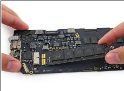
• Lift the free end of the SSD up slightly and pull it straight out of its socket on the logic board.
