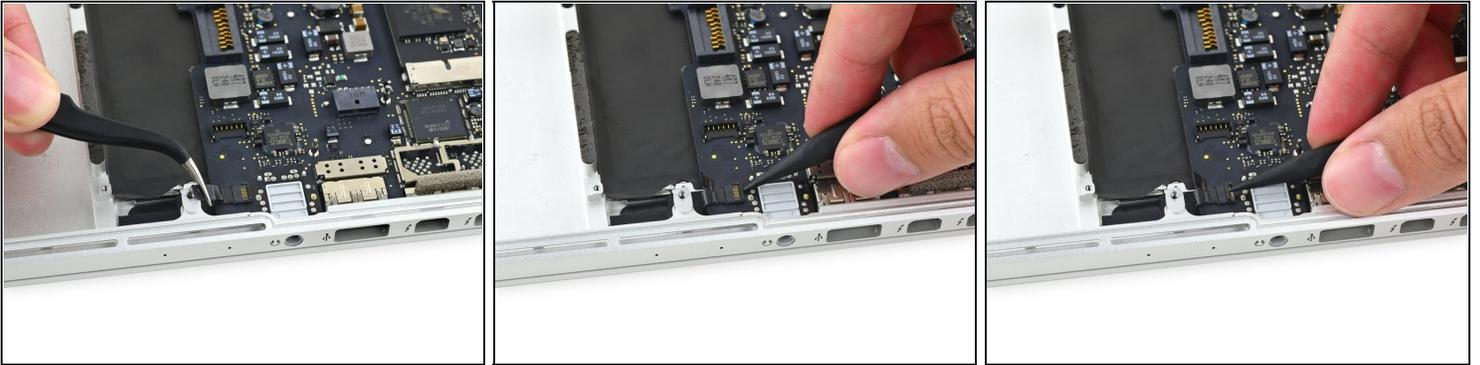
ⓘ If necessary, peel back any tape covering the microphone cable ZIF connector.
