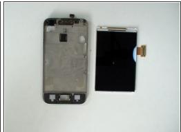
Again by using a plastic tool, separate the LCD display from the middle frame.
