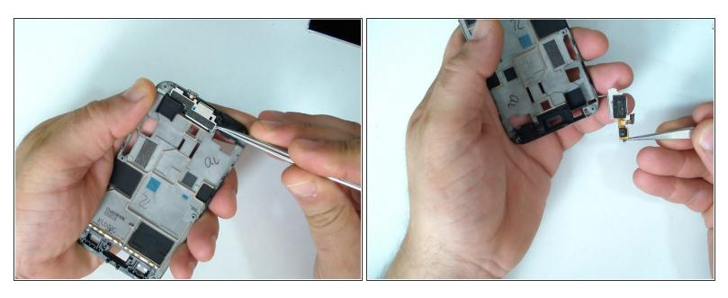
Loudspeaker and light sensor module,
