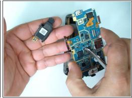
This is the loudspeaker & audio jack connector module.
