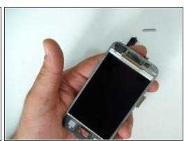
Clean the middle frame and install the LCD display.
