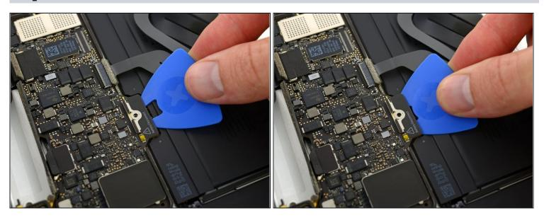
As an added precaution, you may physically disconnect the battery by inserting a battery isolation pick between the logic board and the battery connector.
