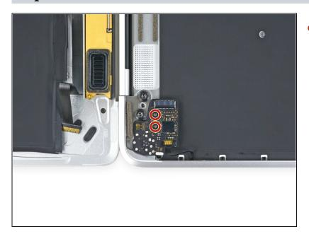
Remove the two 3.2 mm T5 Torx screws securing the audio jack board to the case.
