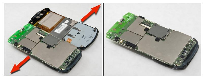
Separate the circuit board from front cover.
