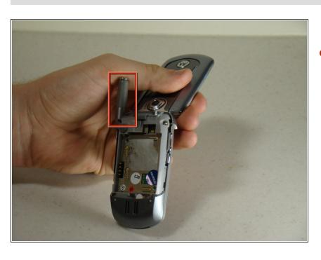
Locate the antenna port on the top of the phone.
