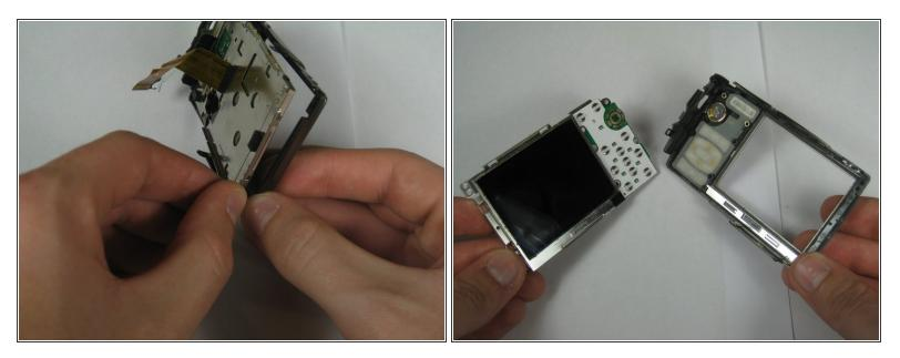
• Push out the LCD screen by pushing on the screen side.
