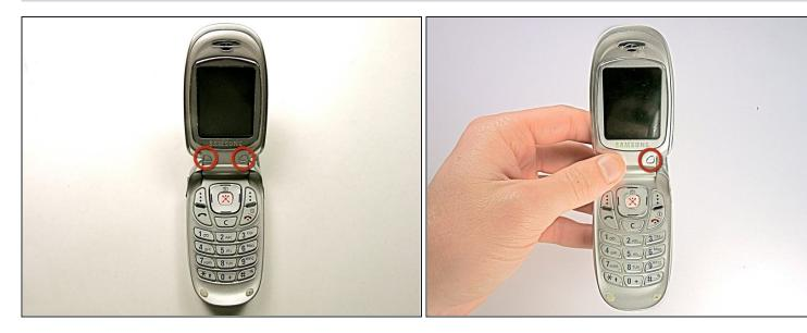
• Remove the plastic coverings at the base of the LCD screen using your fingers.
