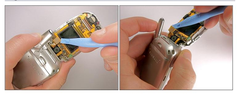
• Use the wedge to detach the connecting wire panel from the LCD display system.
