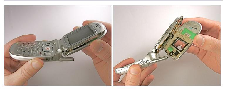
(i) Make sure that the top panel is completely separated from the LCD display around the entire perimeter.
