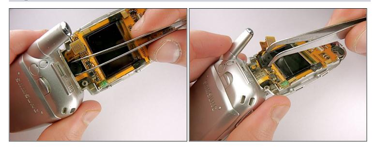
Use the tweezers to remove the camera from the cellphone casing.
