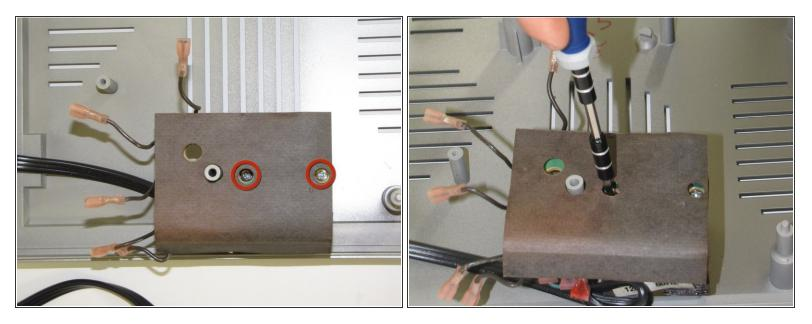
• Remove the two 1.6 inch screws securing the transformer.
