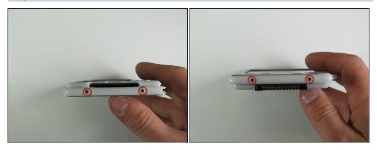
• Remove the four 2.6 mm Philips screws on the top and bottom of the frame.
