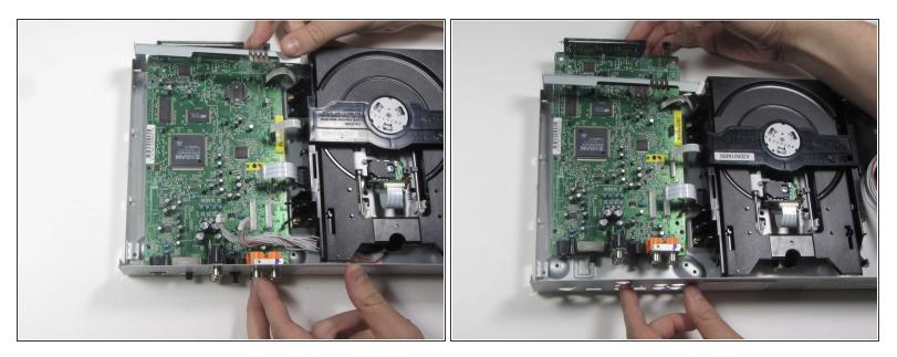
• Push the motherboard forward a few inches to detach it from the casing.
