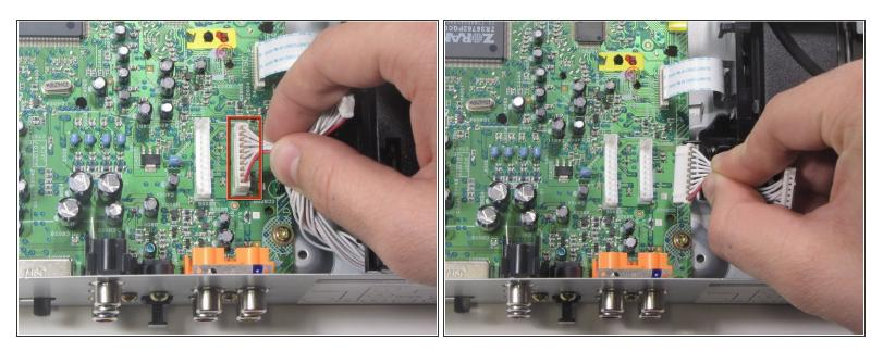
Remove the second of two multipin cables connected to the Left-Side Motherboard (Green) by pulling vertically.
