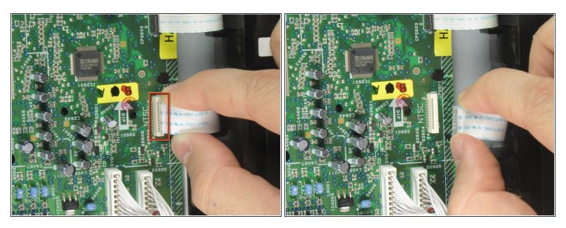
• Remove the first of three ribbon cables on the left hand side of the disc drive by pulling vertically.
