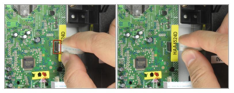
Remove the second of three ribbon cables on the left hand side of the disc drive by pulling vertically.
