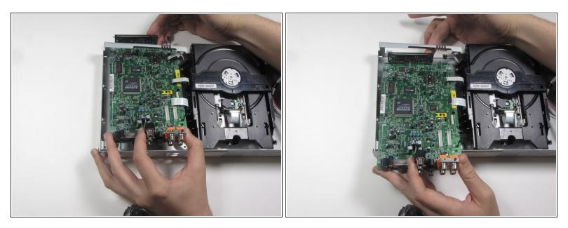
Lift the motherboard from the rear and pull backward (towards you) to remove it entirely from the case.
