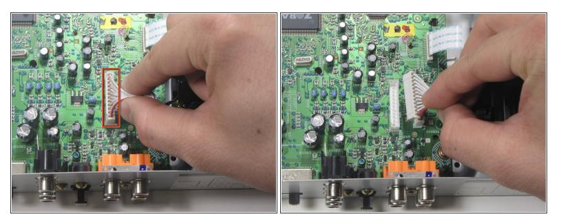
Remove the first of two multipin cables connected to the Left-Side Motherboard (Green) by pulling vertically.
