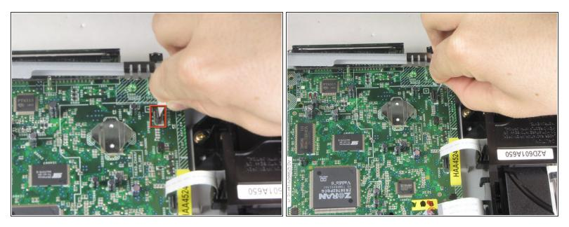
• Remove the third of three ribbon cables on the left hand side of the disc drive by pulling vertically.
