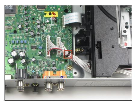
Remove the black tie holding the two rear ribbon cables together by untwisting it.
