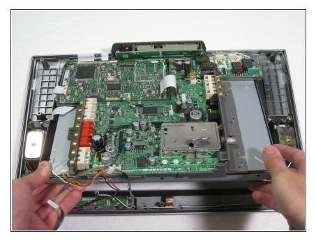
Lift the circuit board/LCD block from the case by lifting the near side of the circuit board and sliding it under the button frame.
