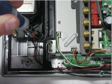
Remove the four 5mm phillips screws attaching the LCD and circuit board to the front case.
