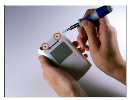
Unscrew the two 7.35mm Torx T6 screws.
