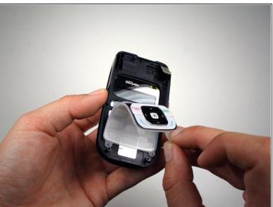
Use your fingers to remove the keypad by carefully pulling from the top of the phone towards the bottom of the phone.
