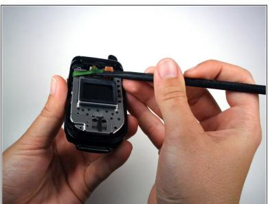
Using the spudger, disconnect the green display cable.
