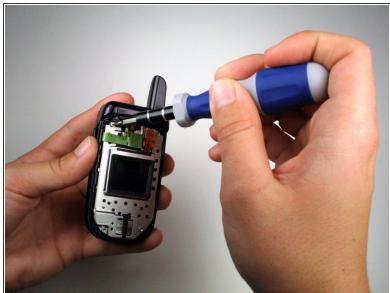
Remove the four 5mm screws on the metal casing using the T6 Torx screwdriver.
