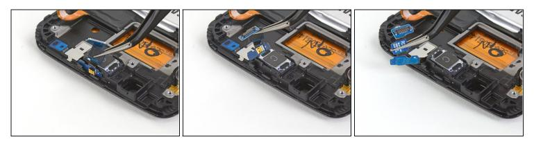
• Lift the earpiece assembly board from its routing channel above the earpiece speaker.
