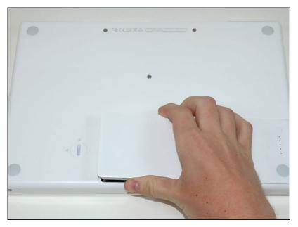
• Lift the battery out of the computer.
