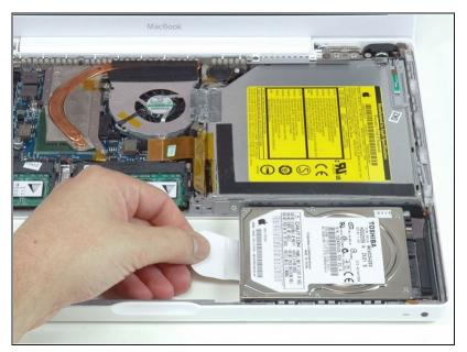
Grasp the white plastic tab attached to the hard drive and pull it to the left, removing the hard drive from the computer.
