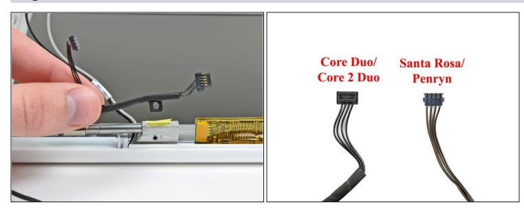
• Remove the inverter cable from the display.
