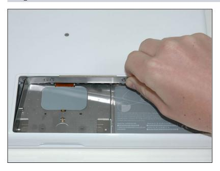
Lift up on L-shaped memory cover, slide it to the right, and lift it out of the computer.
