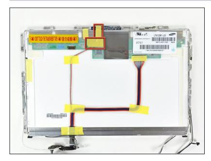
• Remove the two pieces of yellow tape covering the camera cable near the top edge of the LCD assembly.
