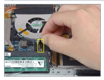
• Disconnect the newly-revealed display data cable. If there is no pull-tab on the top of the connector, it may be helpful to use a spudger to disconnect this connector.
