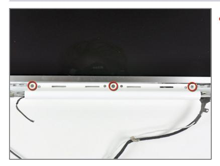
• Remove the three 4.2 mm Phillips screws securing the clutch cover.
