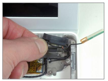
• Lift the right speaker out of its housing and set it to the side.
