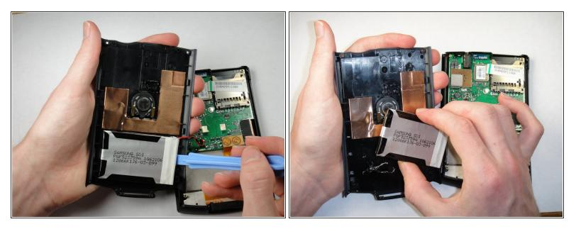
• Use a plastic opening tool to peel the battery pack from the back panel.
