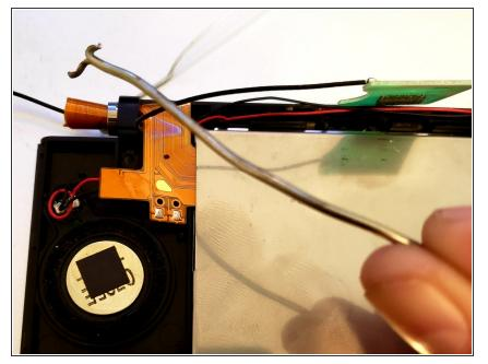
Use a small hook to help curl the leading edge of the ribbon through the display hinge. A piece of solder like this one (shown) works well.
