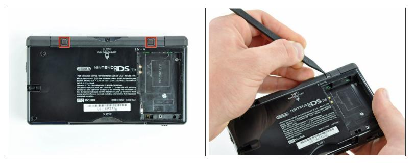
• Use the tip of a spudger to pry both rubber feet off the DS Lite.
