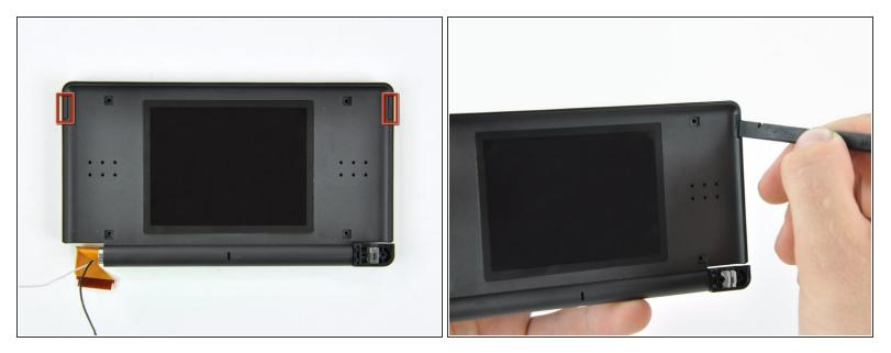
• Use the edge of a spudger to pry both rubber pads out of the front display bezel.
