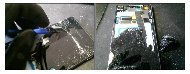
• Continue removing the looser pieces. Use plastic tools, so you don't damage the electronics inside.
