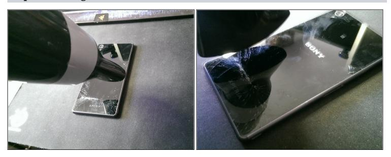
• Start by using a blow-dryer on the hottest setting. Heat the entire backside of the phone, and focus on the edges for a minute or two.
