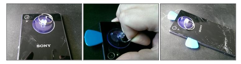
• Use a suction-cup to pull up the back-cover about 1mm. Insert a pick and use a second one to make the opening larger.
