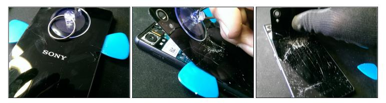
• Use the picks to get the cover off as far as possible. After this, wear gloves and try to pull off the glass. It will break in this step, so be careful for any pieces of sharp glass!
