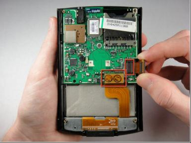
Pull straight up on the ribbon cables located on the bottom right of the motherboard to disconnect them.
