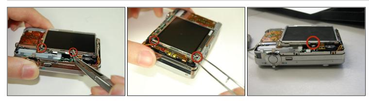
• Use the tweezers to pry the LCD screen off from the openings. There are 5 spots that the tweezers can go in to pry the LCD screen off (see attached pictures).
