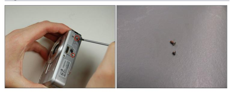
Remove the two back screws on the bottom of the camera on the same side as the LCD screen.
