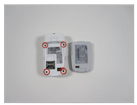
• Remove the 4 (4.7mm) philips head screws.
