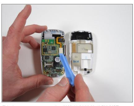
Use an opening tool to gently lift the ribbon wire connection to the screen.
