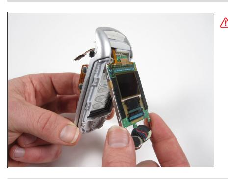
Carefully feed ribbon wire through the phones joint.
