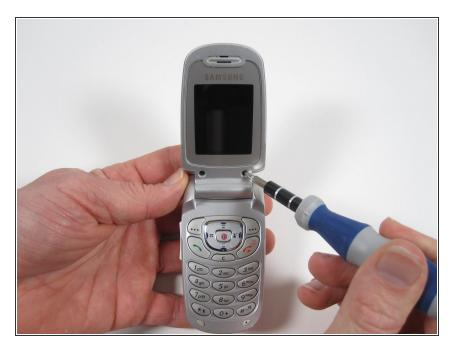
Remove the 2 (5.6 mm) philips head screws with your safety or push pin.
