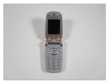
First, remove the 2 silver stickers (as indicated by the circles) with a a safety or push pin to reveal 2 screws.
