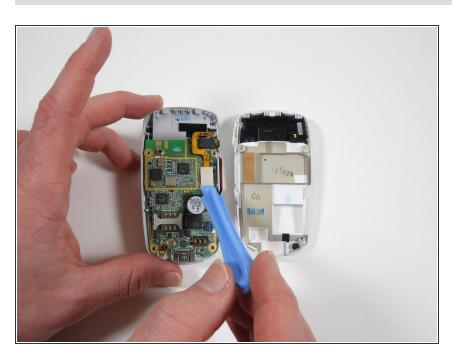
Remove the ribbon wires connecting to the screen using the pry tool.
