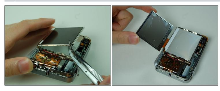
Use tweezers to lift up the LCD screen away from the camera.
