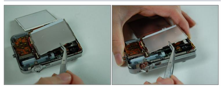
Use tweezers to slowly pry off LCD casing by lifting and moving it off the camera.
