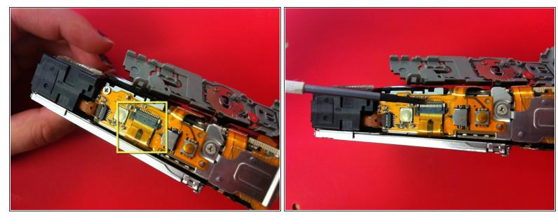
Using the spudger, flip the clip in an upward motion. The clip should remain attached to camera, not removed completely.
