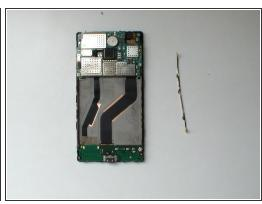
Disconnect the Antenna cable from the Logic board and from the Charging Dock board and remove it.
