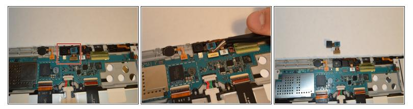
• Use plastic tweezers and carefully detach the rear-facing camera from the motherboard.
