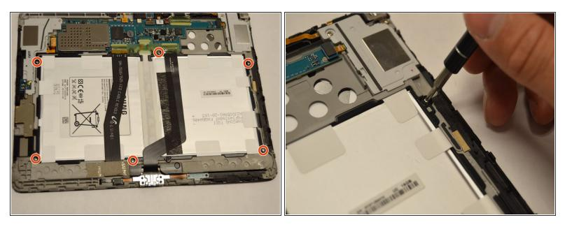
• Remove the six 4 mm Phillips #00 screws that hold the battery in place.
