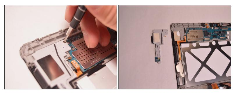
• Remove the Phillips #00 screws from the plastic part holding down the motherboard.
