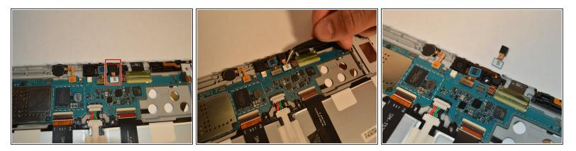
• Use plastic tweezers to carefully detach the front-facing camera from the motherboard.
