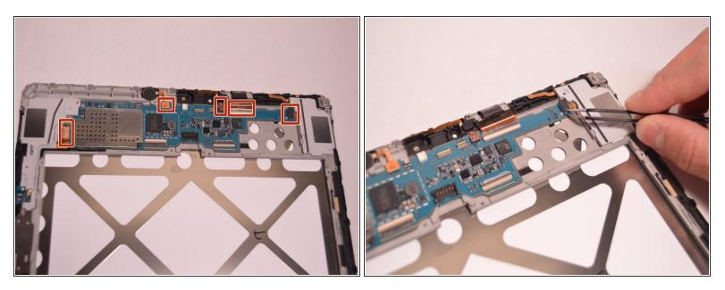
Remove the five ribbon cables holding the motherboard together with a plastic tweezer.
