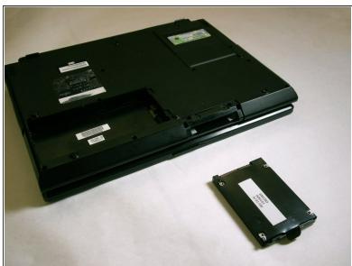
Grasp hard drive sleeve tab and pull out.
