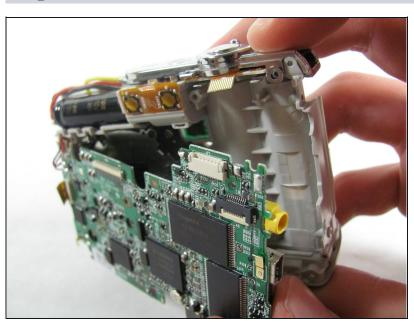
Remove the motherboard from the camera casing.
