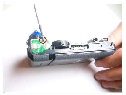
Remove the individual 4mm screw under the top button to release the motherboard from the housing.
