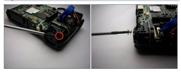
• Remove the big headed 3.5 mm screw that holds the lens in place.
