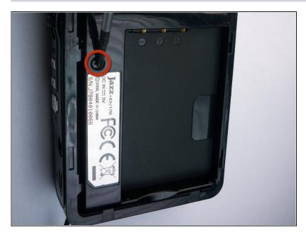
• Remove the 4.5 mm screw located near the battery slot.
