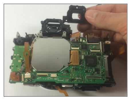
After removing the top panel, you can use your fingers to remove the eye piece from the camera.
